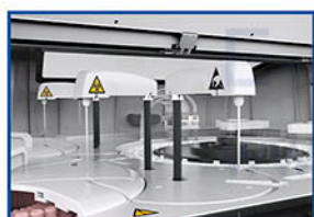
Chemistry Analyzer Module-Sample /Reagent Probe
